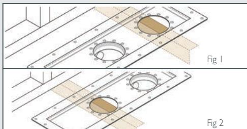
aqua4ma linear has two waste hole positions (Fig 1 & 2). If joists run along the length of the deck, you simply choose the position that will avoid them.
