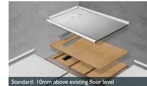
Flooring removed to size of aqua4ma Shower Deck, create a false floor at joist level, add plywood panel to lift shower deck 10mm above existing floor level to allow joining to aqua4ma Floor Panels. Then use aqua4ma 10mm Panels to waterproof all or part of the floor to the same height as the shower deck.
