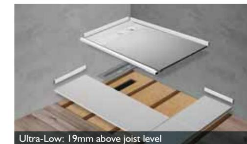
(Additional waterproof floor area at same level) Flooring removed to desired area and false floor created at joist level. aqua4ma linear Shower Deck and 19mm floor panels fitted within the removed floor area.
