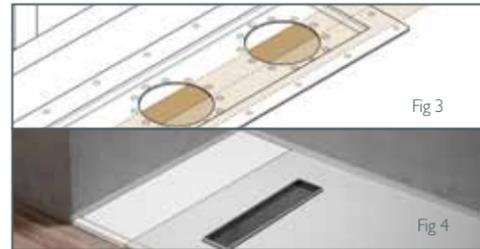
Should joists run across the deck (Fig 3) and obstruct the waste location, a wedge shaped extension panel is available (Fig 4). This 250mm trim-to-fit panel solvent welds to the base so it can be moved away from the obstructing joist whilst maintaining the fall to ensure efficient drainage.
